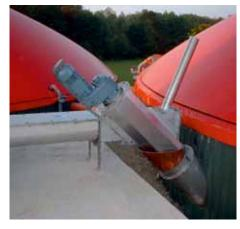
Base frame screw and fermenter screw model 360 for floor grade input We tailor our conveyor systems to a site's
